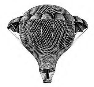
fire, may be raised or lowered to regulate the draught. The air fed to the fire is admitted through a perforated truncated cone, and a similar cone, but inverted, is employed to conduct the heated air to the balloon.
